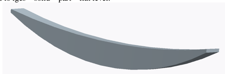
Fig.2 Model of mono composite leaf spring
