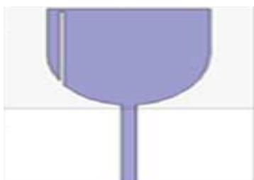
Fig.1.Model of WiMAX rejection band
