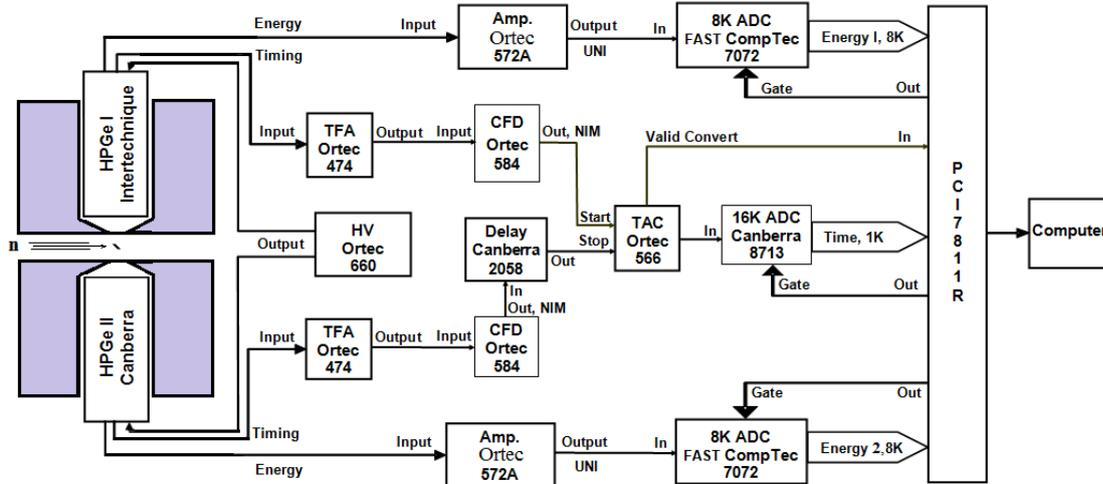
Fig. 1. The experimental system for gamma-gamma coincidence measurement [9]
