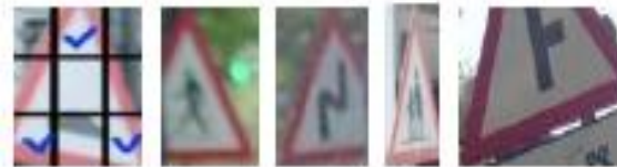
Fig. 3: Using Corners for identifying triangular borders.
