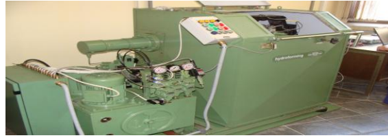
Figure 4: Experimental analysis device of tube hydroforming process
