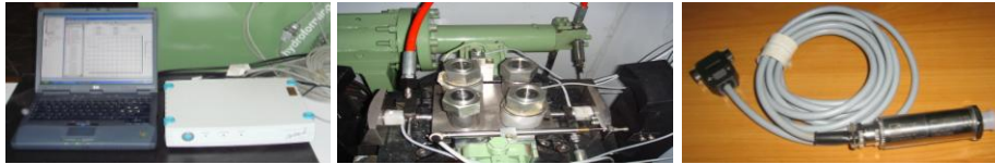
Figure 5: Measuring amplifier device, Spider 8, P3MB – Fluid pressure sensor in the tube
