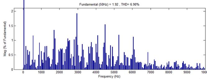
**Figure 8(b). Harmonic spectrum for hysteresis controller (R=96Ω,L=30mH)**
