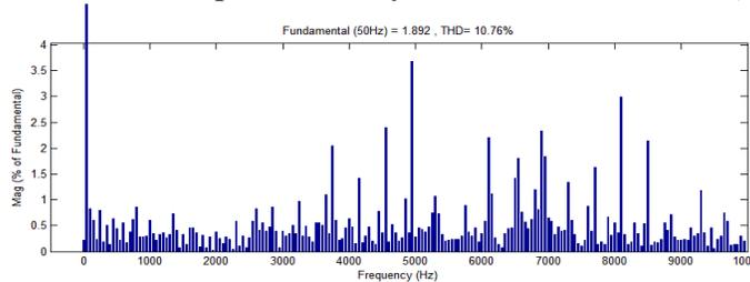
**Figure 8(c). Harmonic spectrum for hysteresis controller (R=47Ω,L=15mH)**
