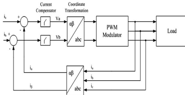
**Fig. 5. The block diagram of PI current controller.**
