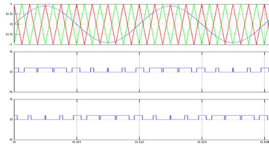
Figure 2. Phase Shifted PWM (PS-PWM)
