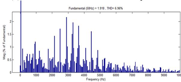
**Figure 8(a). Harmonic spectrum for hysteresis controller (R=96Ω,L=35mH)**
