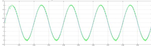
**Figure 7(b). Reference current waveform for hysteresis controller**
