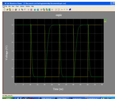
**Figure 4.** Spice simulation showing the glitch minimization
